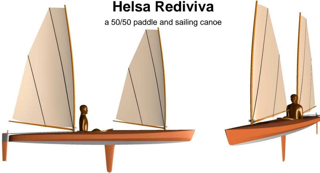
The background of this design is to create a modern boat with the same characteristics as my own "Helsa", designed by Carl Smith, built in 1882. It is a "50/50" paddle and sailing canoe, probably the most versatile type of boat that also can be easily transported on a car roof. "50/50" means a sailing canoe design which is equally happy being paddled with a double kayak paddle or sailed. Both aspects work really well.
