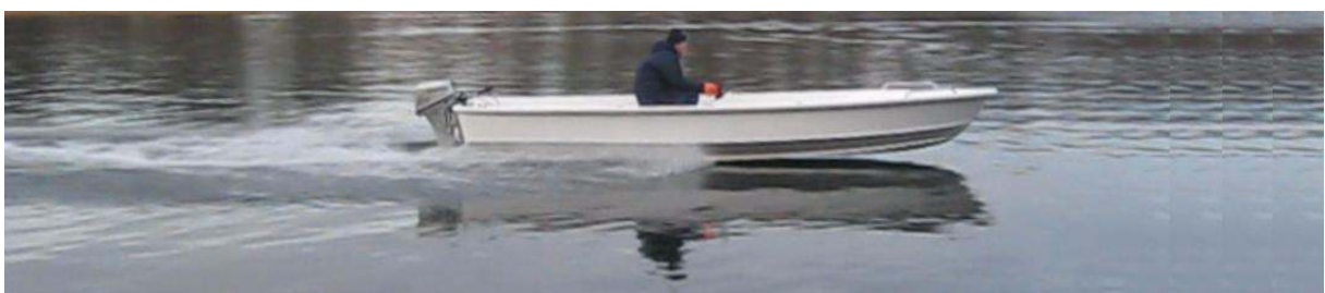
Test 081128 with W 330 with midship interceptor at 19 knots with 8 horsepower
